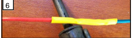
6. Apply heat to HSS to insulate joint
