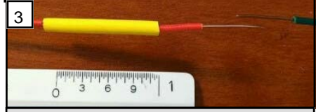
3. Heat Shrink sleeving to cover joint
