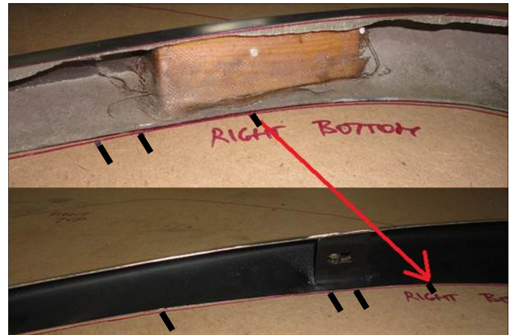
Only the last bracket location was slightly adjusted as shown in photo below (75mm from the inner edge of the over-rider).
